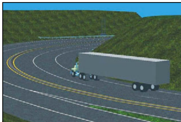
Visualizations can also be used to show alternative scenarios. In this instance, the visualization demonstrates that a properly loaded tractor-trailer could negotiate the turn at speeds significantly higher than those posted proving that the shifting load, not speed, was the causal factor in the accident.
