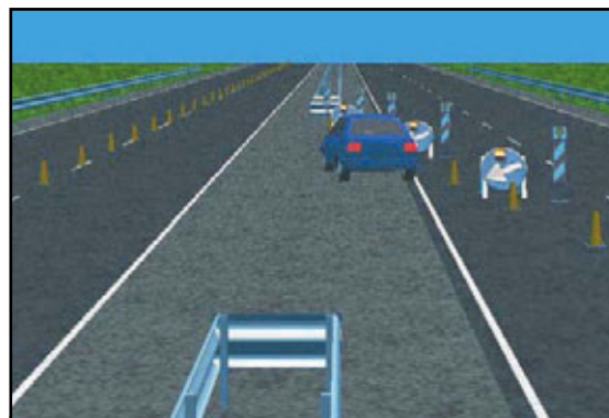
This visualization of a highway construction work zone shows that the driver of the vehicle obeyed the temporary traffic control devices that sent him directly into the unmarked barrier protruding into his lane, resulting in two fatalities. The airman was later exonerated of all charges related to the crash.
